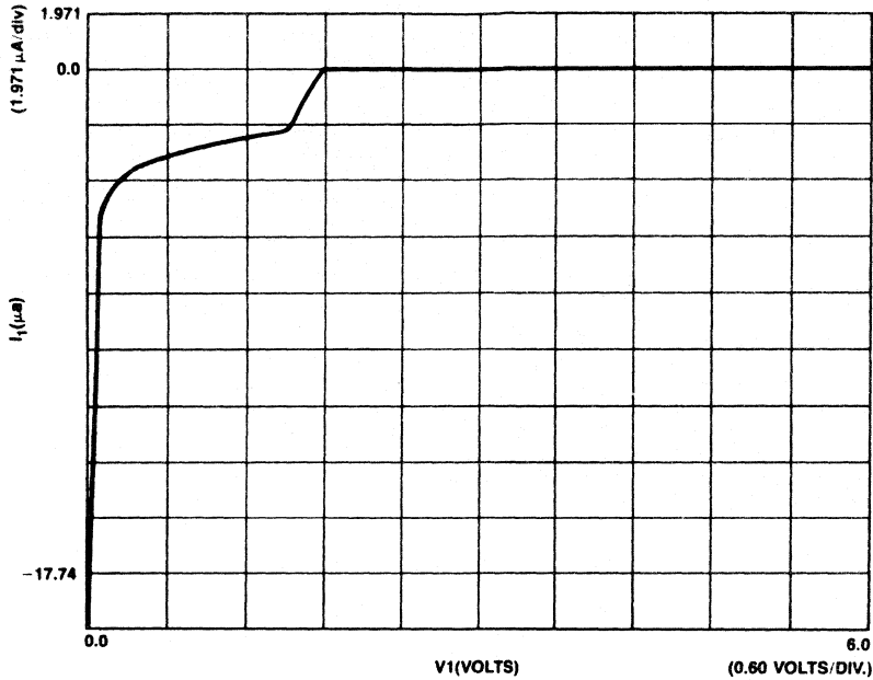
Figure 5. Input Current vs Input Voltage Characteristics of I/O Pins
